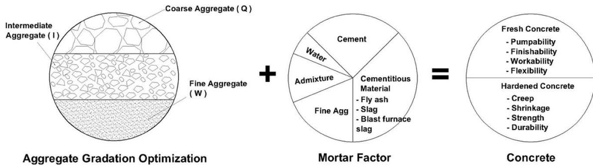
Fig. 4. Efficiency concrete flowchart
